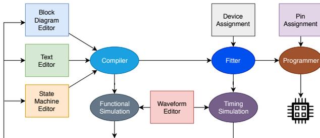
Figure 6. Design flow using Quartus.
