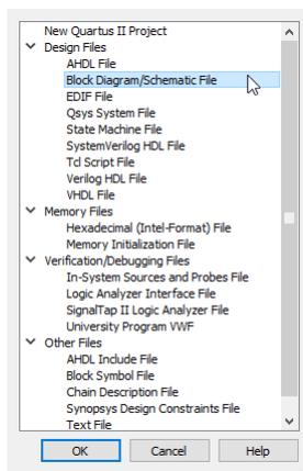
2. Highlight **Block Diagram/Schematic File**, and click **OK**. The schematic entry window will appear on the working space as shown.
