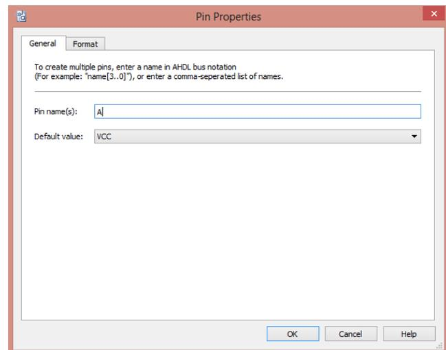
**Figure 17.** Naming input pins.
